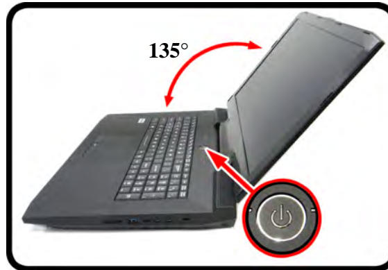
Figure 1 - 1 - Computer with AC/DC Adapter Plugged-In/Opening the Lid/LCD
